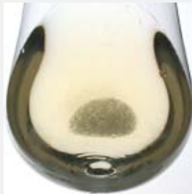
Fig. 3.7. Shows calcium-tartrate crystals in a white wine. This is not a manufacturing defect but more of a cosmetic irritant. It is caused through attraction of various acids and calcium along with cold storage conditions.
